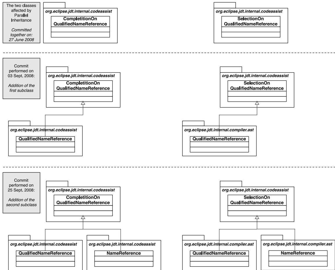
Fig. 6. An identified Parallel Inheritance instance: the pair of classes CompletionOnQualifiedReference and SelectionOnQualifiedReference from ECLIPSE JDT.
