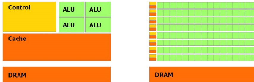
FIGURE 3.2 – Architecture CPU et GPU Kirk et Wen-Mei [2016]
