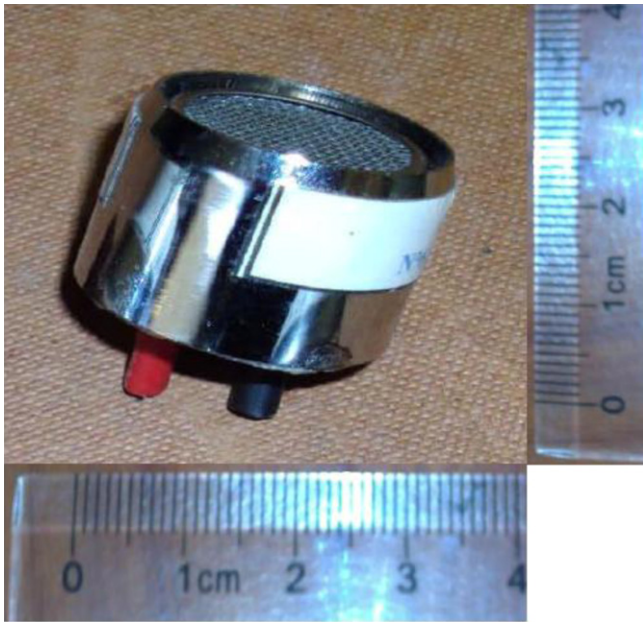
Fig. 3. Prototype of Au-Porous a-Si 0.70 C 0.30 /Si(p) humidity sensor.
