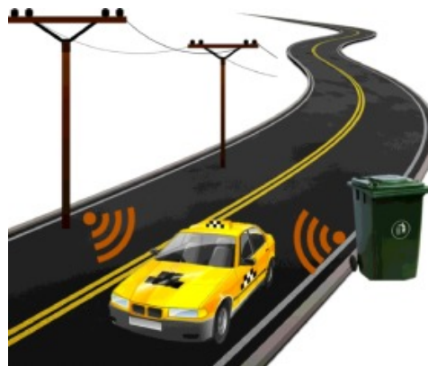
Figure 3.9: Dataxis proposed scenario: Opportunistic data exchange between taxi cabs and IoT nodes.
