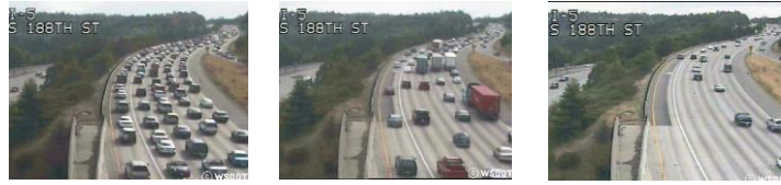
Figure 2.13 : Three images from UCSD illustrating traffic conditions categorized as Heavy, Medium and Light.
