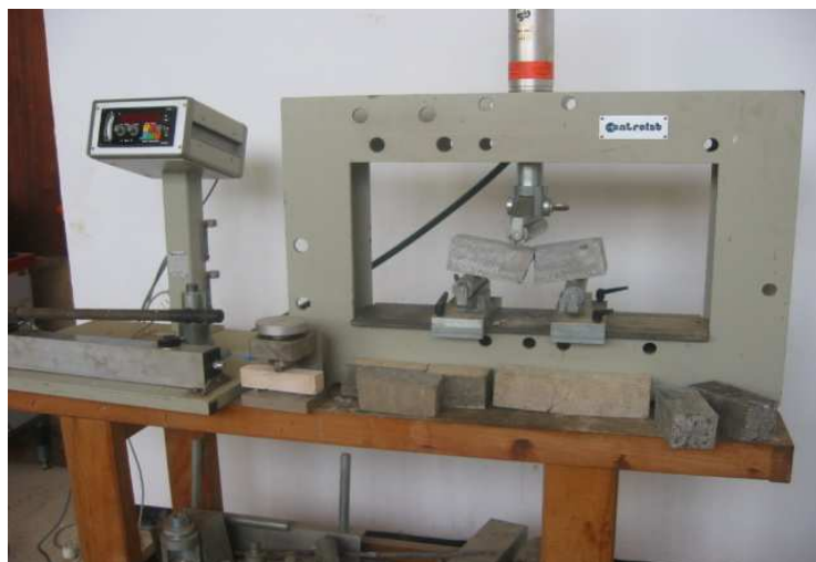
Figure 9-7: Portique universelle asservie (Controlab)
