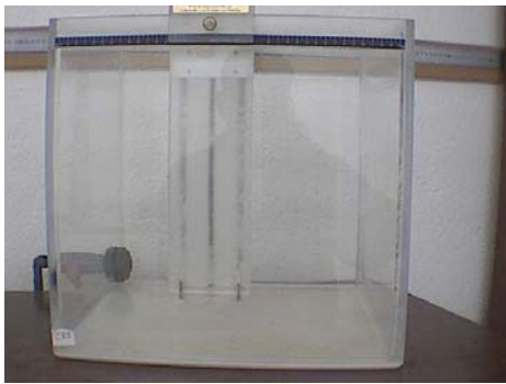
(a) Fantôme MEDTEC (Irradiation verticale)
