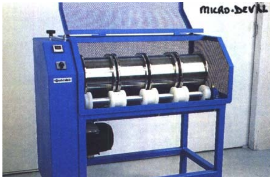
Figure II.4 Machine Micro Deval.
