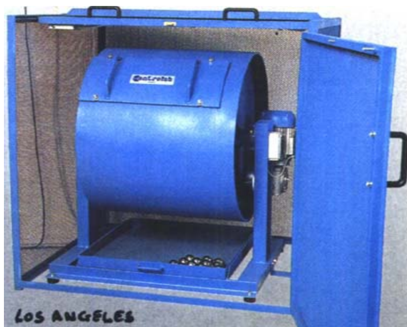
Figure II.3 Machine Los Angeles.
