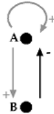
Figure 2.15: Regulon scheme. Grey arrows are activatory (+) whereas the black one is inhibitory (-). A activates the formation of B and its own formation ( self - catalysis ), whereas B inhibits the formation of A.
