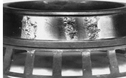
Figure 2.8 Ecaillage de fatigue.
