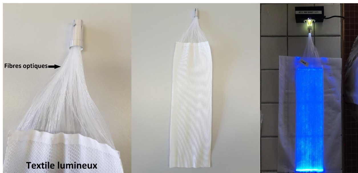
Figure II. 4 Image du textile lumineux (dimensions : 30x10 \text{cm}^2 )
