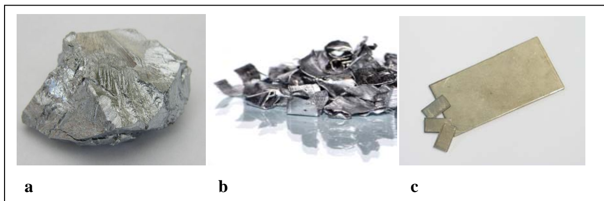
Figure I.1 : Aspect du chrome pur (a), vanadium pur (b) et niobium pur (c).
