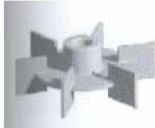
Figure I.7. Turbine de Rushton
